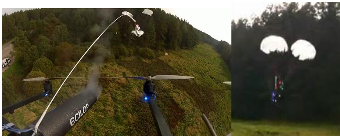
Figure 54 - The Ecilop deploying its parachute (left), and landing under parachutes (right). Images by Aleksey Zuitsevsky.
