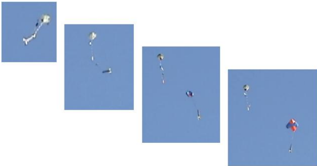
Figure 16 Recovery Package Consisting of Dual Deployment via Tender Descender
