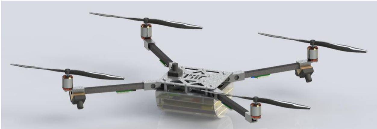
Figure 32 The Current Design of Quadrotor and Science Sensor Suite Configuration
